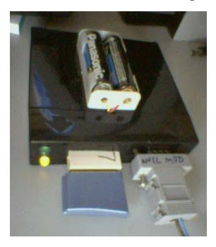
Uploder working. The yellow LED indicates it is saving something (in this case, it is uploading data to the cartridge).
