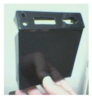
The box: I picked up and old 3 1/2" floppy disk box and drilled some holes on it.
