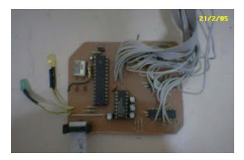
Fully assembled PCB. Note the RS232 flat cable at bottom left of the PCB. I took this cable from an old PC mainboard.
