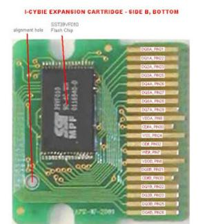
The SST chips are quite cheap and if you have good soldering skills, a magnifying glass and a steady hand you can populate the cartridge yourself. There are some SMD soldering kits in the marked to help you, if you need. The radio and TV repairs guys
